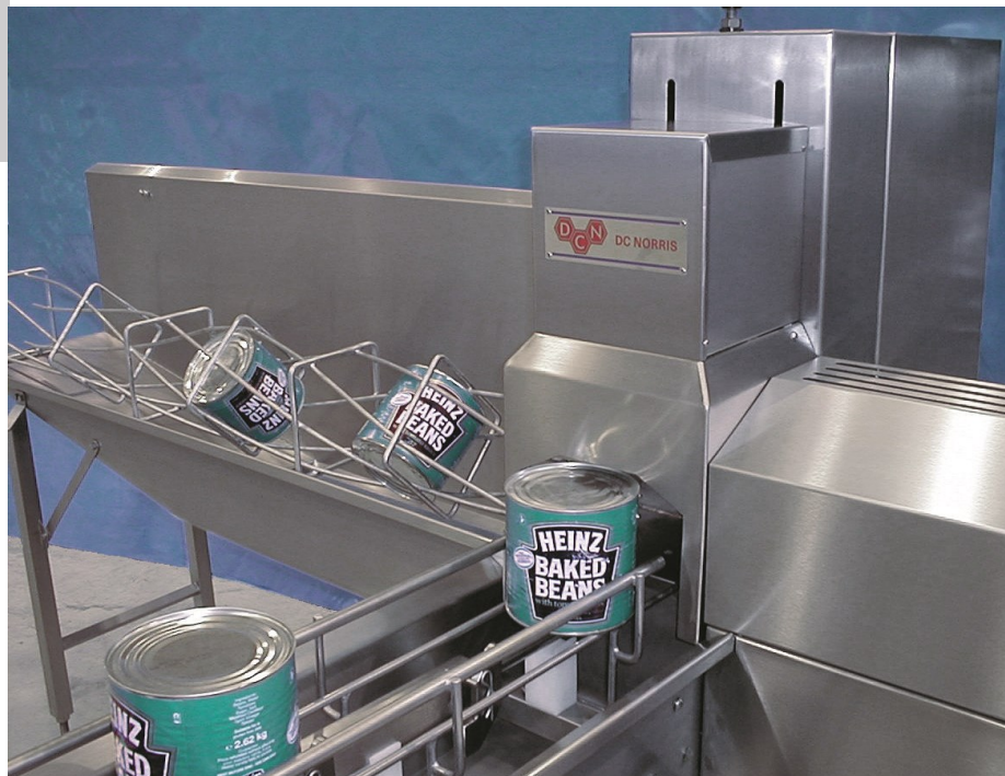
Model shown above includes: Infeed Conveyor, Wash/Dry Tunnel & Can Crusher
