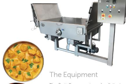
The Bratt Pan comprises of a flatbed, rectangularshaped vessel with a jacket on the underside for heating the product. Liquid draw-off valves are provided front and rear, and the vessel is supplied with hinged covers to retain heat and minimise steam emission.
