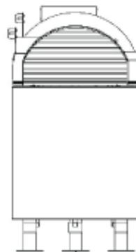
CAN BE ADJUSTABLE FOOT, LOAD CELL PLATE OR TO SUIT CUSTOMER INSTALLATION
